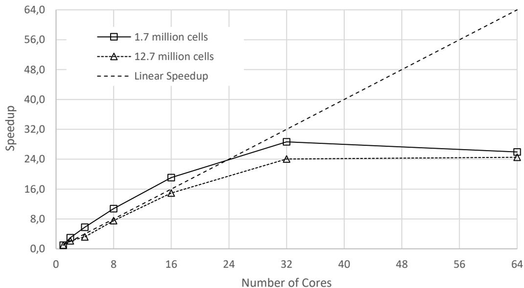
Figure 7 - Speedup for two mesh densities, considering a single node.
