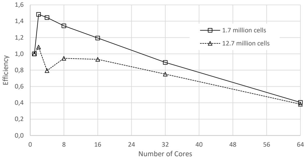
Figure 8 - Efficiency for two mesh densities, considering a single node.
