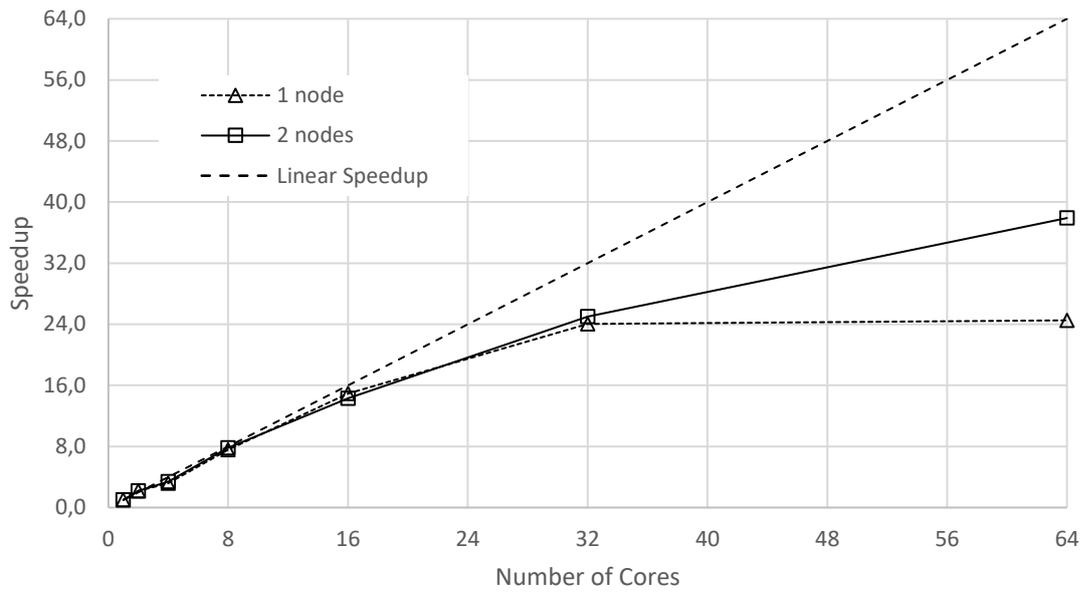
Figure 9 - Speedup using one and two nodes.
