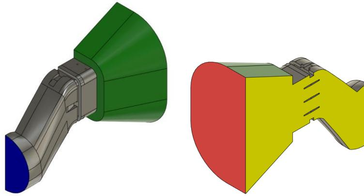
Figure 2 - Interior of the airvent with inlet (blue), outlet (red) and symmetry (yellow) conditions.
