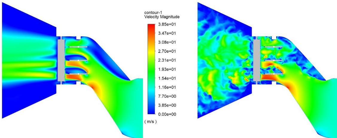
Figure 12 - Flow velocity for (left) steady-state RANS and (right) flow time 0.25s with DES model.
