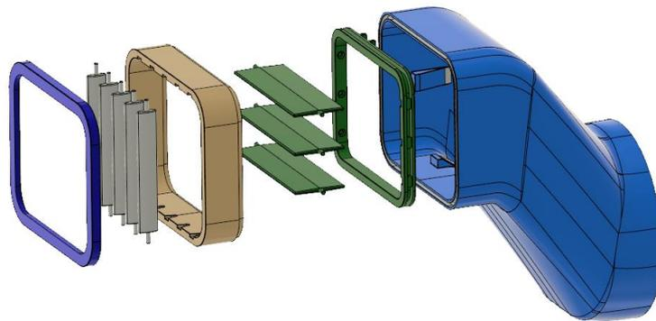
Figure 1 - Geometry of the airvent.
