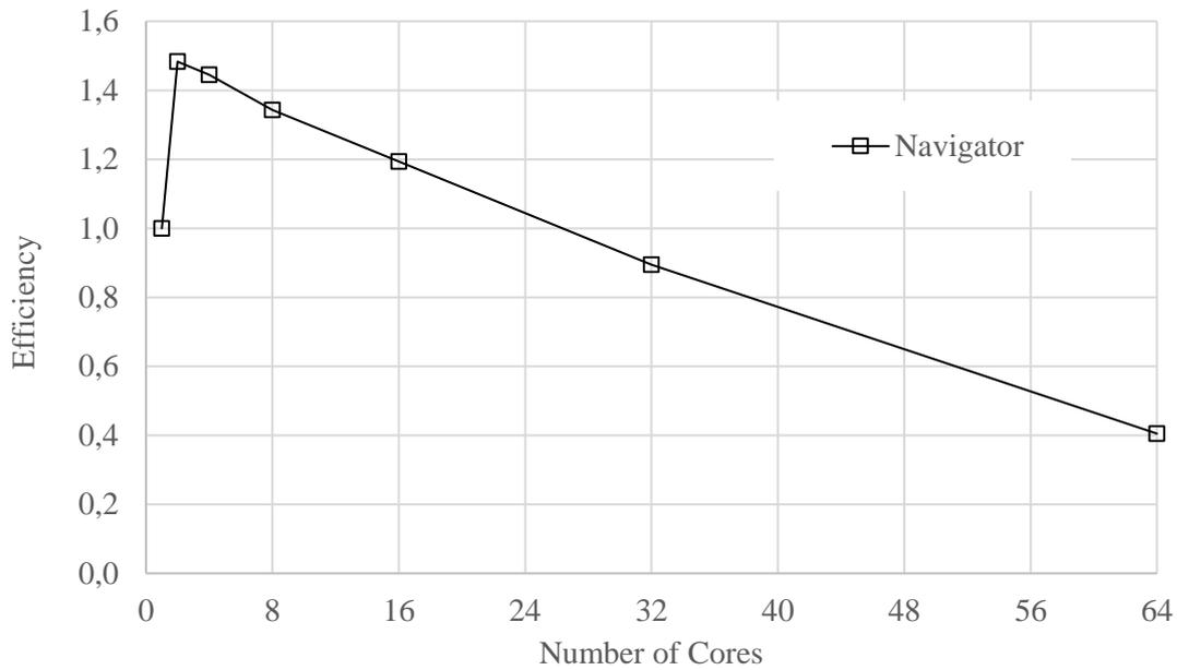
Figure 6 - Efficiency for a 1.7 million cell mesh, considering a single node.
