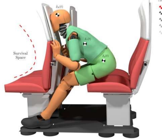
Fig. 2 - Injury prevention test - table down
