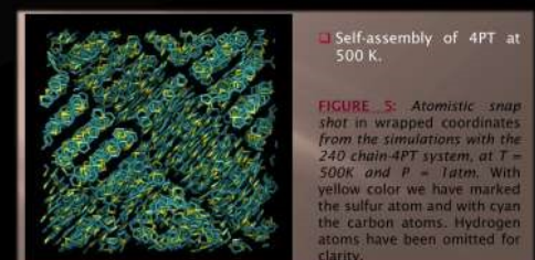
FIGURE 5. Atomistic snapshot in wrapped coordinates from the simulations with the 240 chain-4PT system, at T = 500 K and P = 1 atm. With yellow color we have marked the sulfur atom and with cyan the carbon atoms. Hydrogen atoms have been omitted for clarity.
