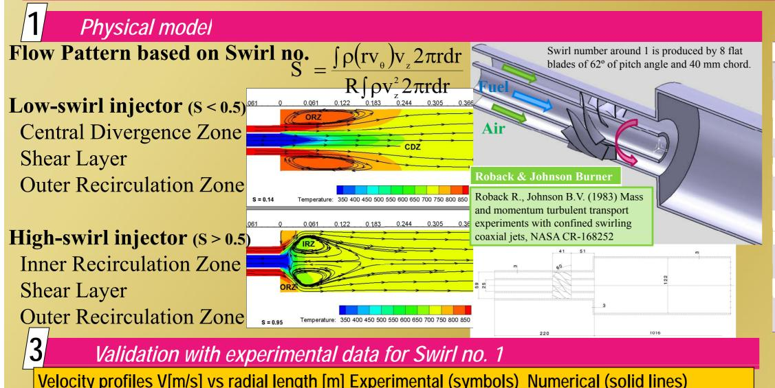
Velocity profiles V[m/s] vs radial length [m] Experimental (symbols) Numerical (solid lines)
